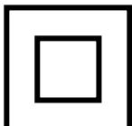
In a double-insulated appliance, two systems of insulation are provided instead of earthing. The symbol (square within a square) may also be used on the product. No earthing means is provided on a double-insulated appliance, nor should a means for earthing be added to the appliance.
