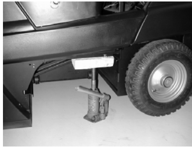
Intake point for the jack (rear wheels)
