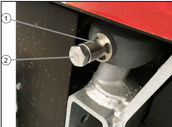
Figure: Variant B with long locking pin
