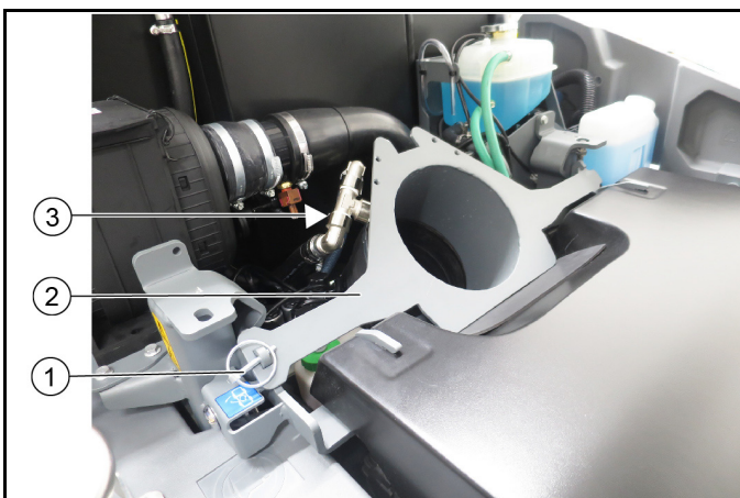
Figure: Sweeping system with changing carriage (shown without suction mouth)
